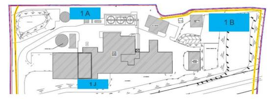
Figure 3.2 Three alternative locations considered for tank farm
