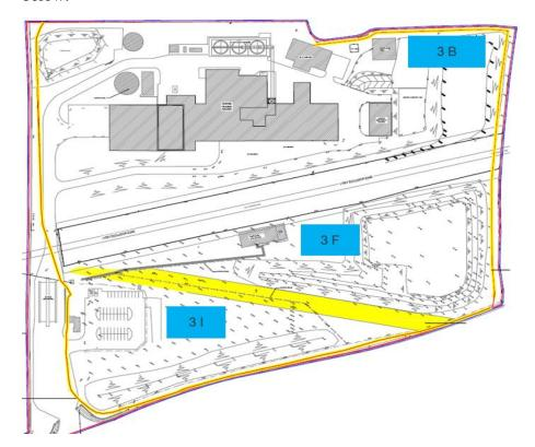
Figure 3.4 Three alternative locations considered for Bottom Ash Storage Building
